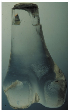
Fig. 5: The first distal femur acrylic prosthesis with a broken stem in Vienna 1964
