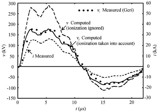
Fig. 10. Comparison with measured transient potentials of a horizontal electrode.
