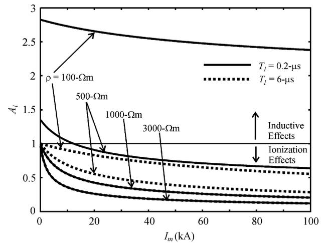
Fig. 15. Impulse coefficient  $A_i$  for current pulses with front times  $T_1 = 0.2 \mu\text{s}$  and  $T_1 = 6 \mu\text{s}$  in case of a single rod (12 m long, 16-mm diameter,  $E_c = 300 \text{ kV/m}$ ).
