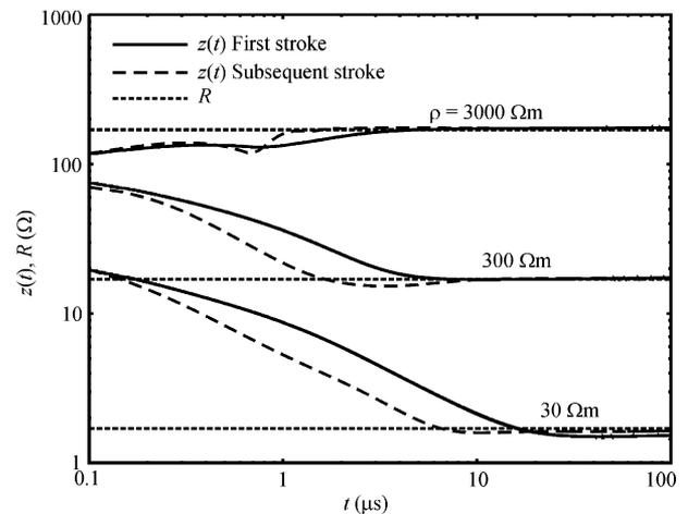
Fig. 8. Transient impedance  $z(t)$  and power frequency resistance  $R$  for the 30-m-long electrode in Figs. 3, 5, and 7 (ionization is ignored).
