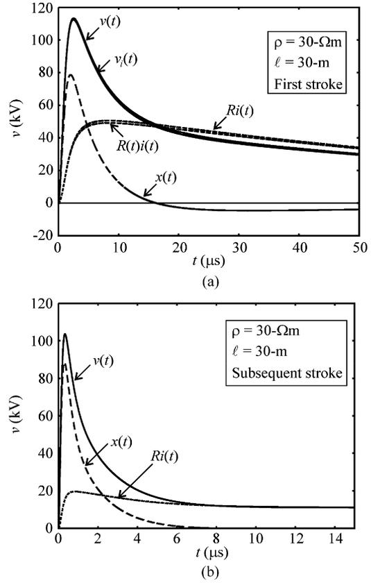
Fig. 3. Very conductive soil and long electrode.
