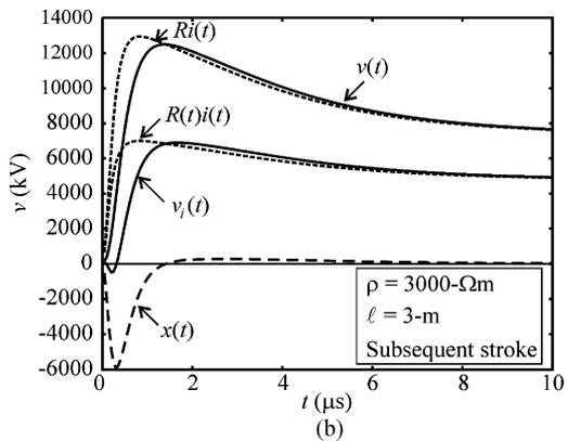
Fig. 6. Very resistive soil and short electrode.
