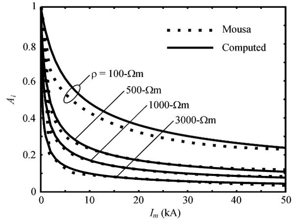
Fig. 12. Comparison with measured impulse coefficient.
