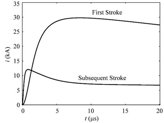
Fig. 1. First and subsequent return stroke currents.
