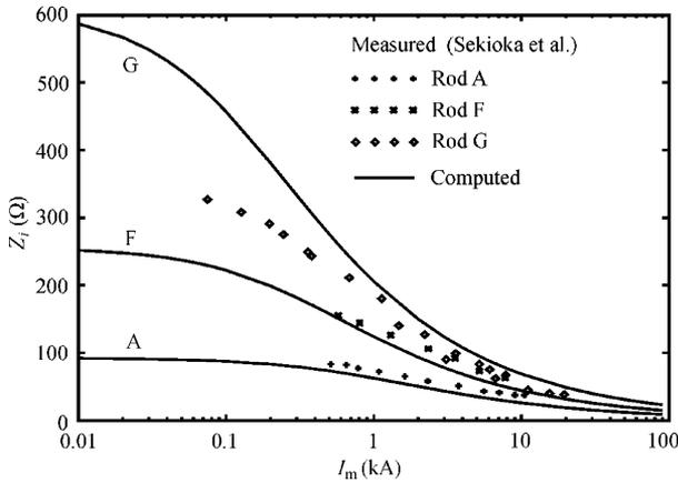
Fig. 11. Comparison with measured impulse impedance.
