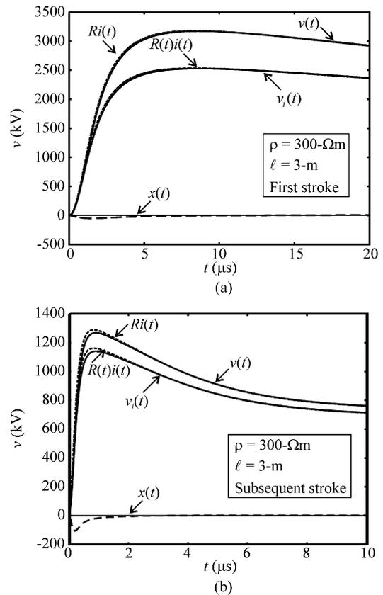
Fig. 4. Resistive soil and short electrode.
