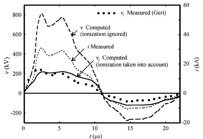
Fig. 9. Comparison with measured transient potentials of a vertical electrode.
