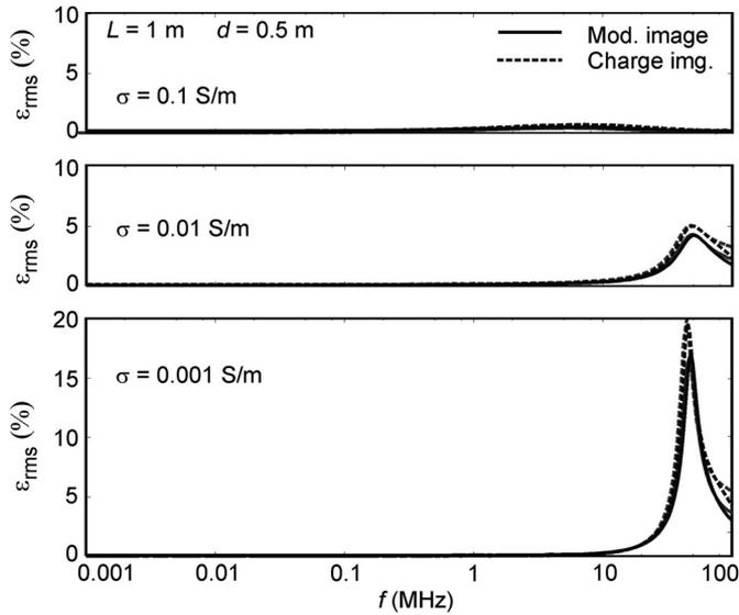
Fig. 4.  $\epsilon_{\text{rms}}$  error for current along the 1-m conductor buried at 0.5 m. Black line—voltage generator excitation. Gray line—plane-wave excitation.
