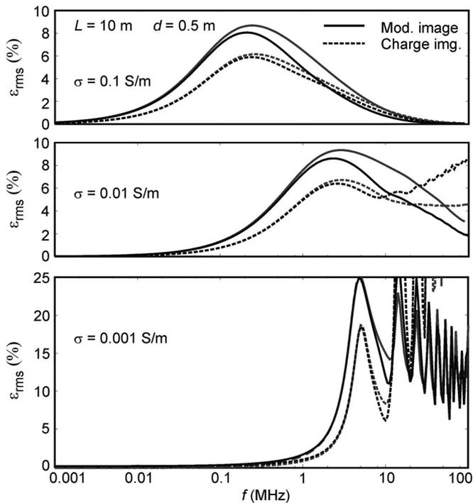
Fig. 5.  $\epsilon_{\text{rms}}$  error for current along the 10-m conductor buried at 0.5 m. Black line—voltage generator excitation. Gray line—plane-wave excitation.
