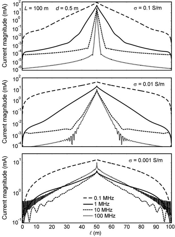
Fig. 2. Current distribution along the 100-m-long wire for antenna type excitation—serial voltage generator 1 V (RMS) at the central point of the wire.
