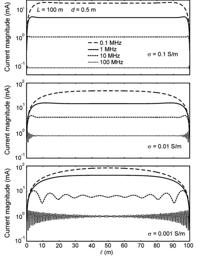
Fig. 3. Current distribution along the 100-m-long wire for scatterer type excitation—illumination by plane wave with 1-V/m electric field tangential to the surface of the wire.
