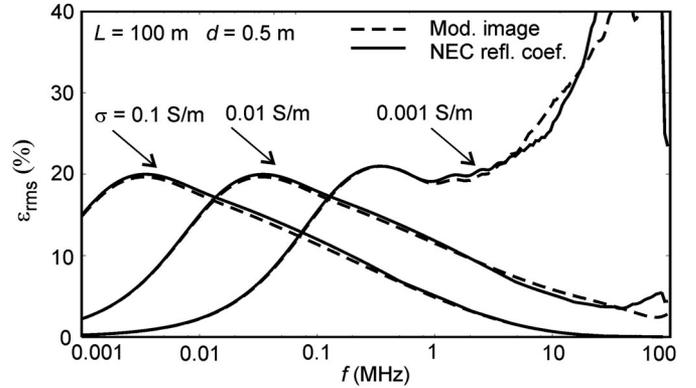
Fig. 11. Comparison of the error for current with NEC for the 100-m-long wire.
