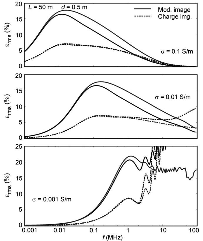
Fig. 6.  $\epsilon_{\text{rms}}$  error for current along the 50-m conductor buried at 0.5 m. Black line—voltage generator excitation. Gray line—plane-wave excitation.
