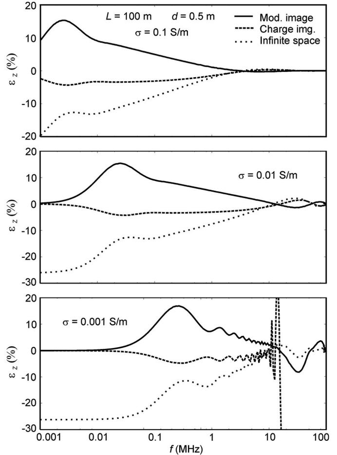
Fig. 8.  $\varepsilon_z$  error for impedance of the 100-m conductor at  $d = 0.5$  m for different soil conductivities.
