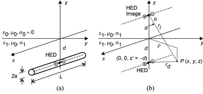
Fig. 1. Illustration of the coordinate system and the position of the buried horizontal wire. (a) Original problem. (b) Image model: HED and its image in unbounded conducting space with the characteristics of earth ( $\varepsilon_1, \mu_0, \sigma_1$ ).
