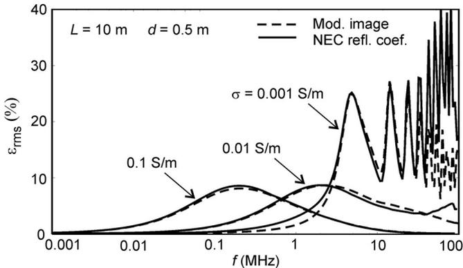
Fig. 10. Comparison of the error for current with NEC for the 10-m-long wire.
