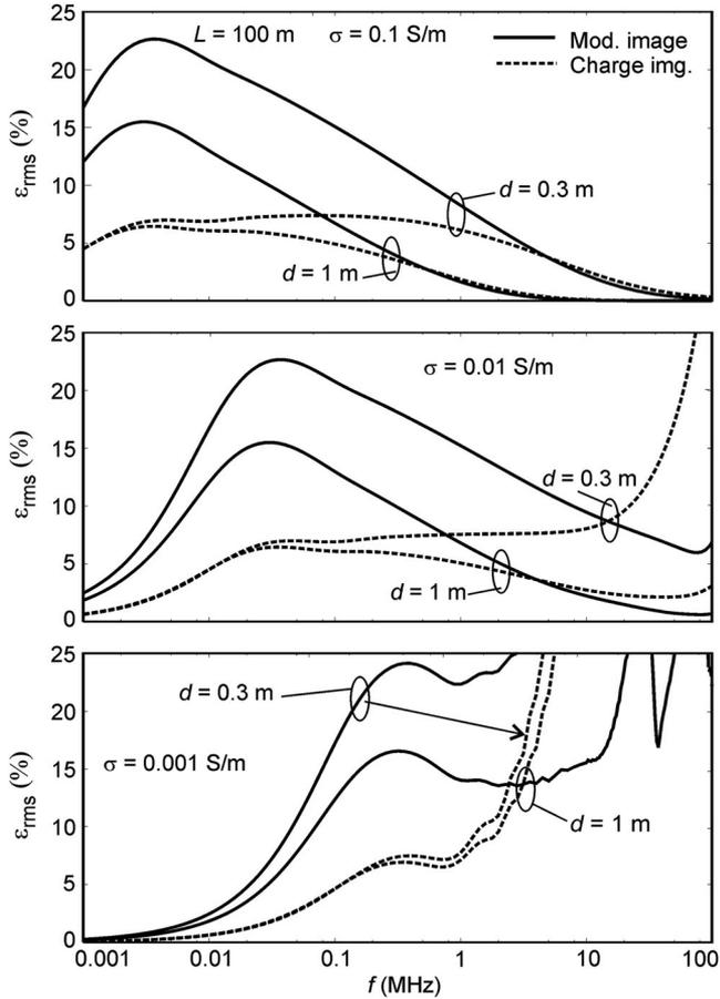
Fig. 9. Error for current along the 100-m conductor at depths of burial  $d = 0.3$  m and  $d = 1$  m for different soil conductivities.
