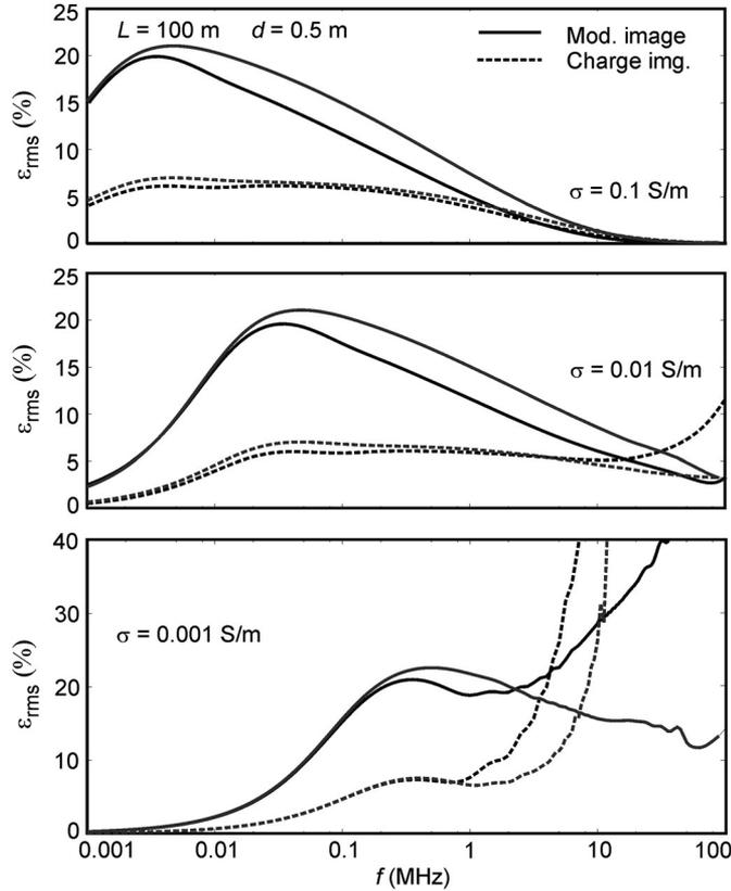
Fig. 7.  $\varepsilon_{\text{rms}}$  error for the current along the 100-m conductor buried at 0.5 m. Black line—voltage generator excitation. Gray line—plane-wave excitation.
