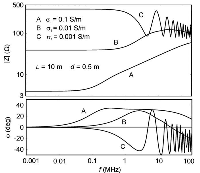
Fig. 12. Modulus and phase of the harmonic impedance at the terminals of the serial voltage generator at the wire's middle point.
