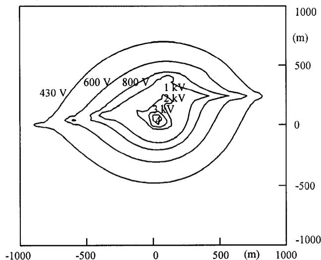
**Figure 10: Potential contours and zone of dangerous influence on telecommunication installations around 110/35 kV transformer station.**
