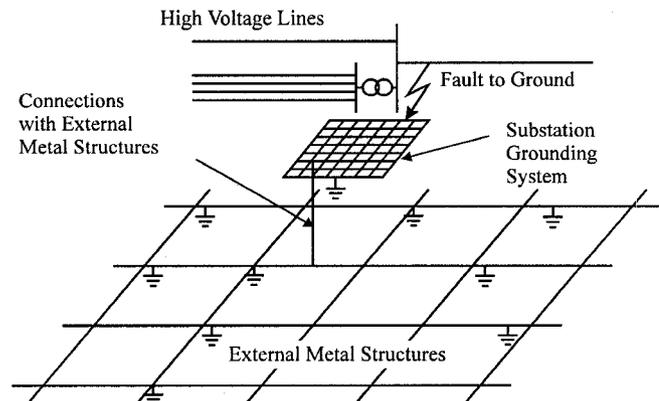
Figure 1. Grounding system of an urban high-voltage substation (adapted from [9]).
