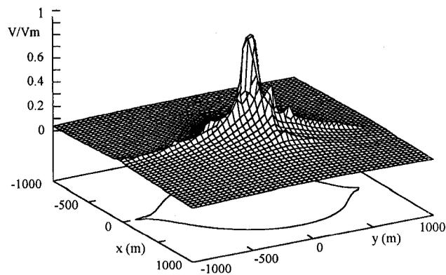
**Figure 9: Earth potential distribution around 110/35 kV transformer station with grounding system connected to uncoated metallic sheathed high-voltage underground cables.**
