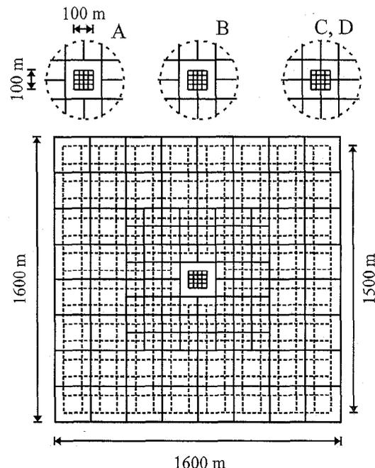
Figure 4. Substation ground grid and two external metal structures.
