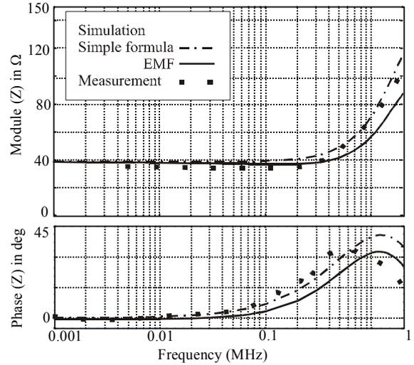
Figure 2: Measurement and simulation of frequency dependent impedance of 16 meters vertical rod electrode.
