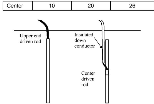
Figure 9. Upper end and center driven rods.
