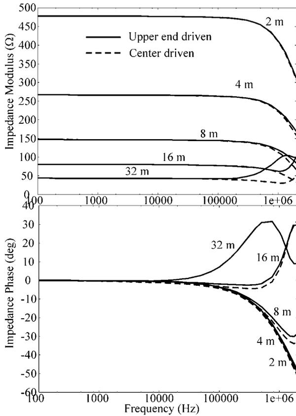
Figure 8. Impedance of ground rods in soil with  $\rho = 1000 \Omega\cdot\text{m}$ .
