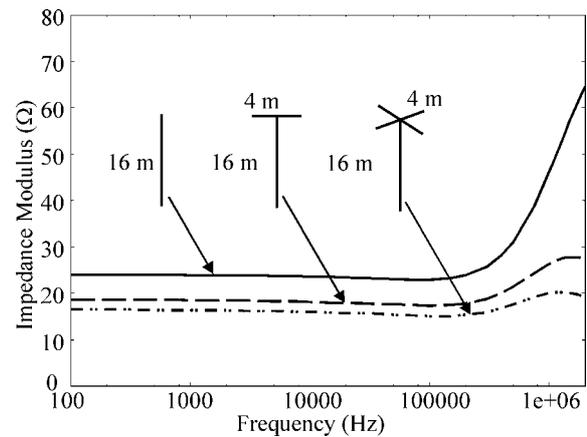
Figure 10. Improved HF impedance of ground rods in soil with  $\rho = 300 \Omega\cdot\text{m}$ .
