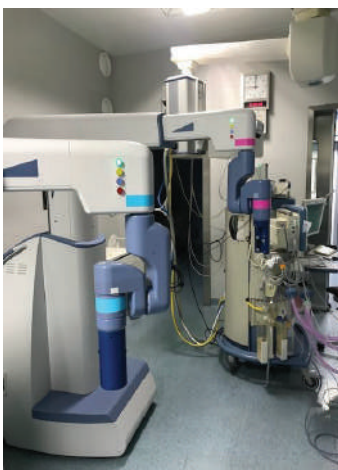
Figure 1a. and b. – Open cockpit platform and two (out of four) robotic arms (which can be easily moved around the operating room).
